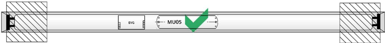
When installing the MU05 leave a distance of at least 10cm to the bulb holders!
