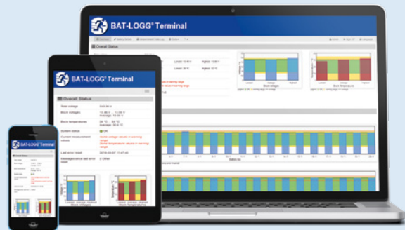
The web interface of the BAT-LOGG® Software with access via notebook, tablet or smartphone.
