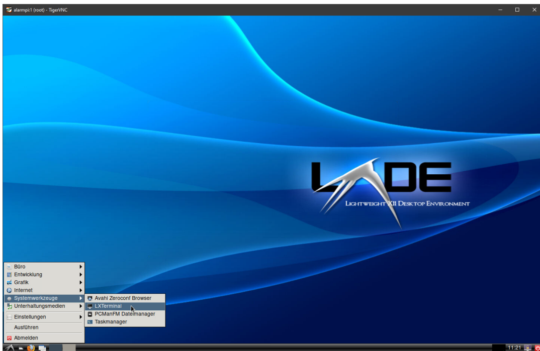
Figure 62 Start terminal on CPC1/2
